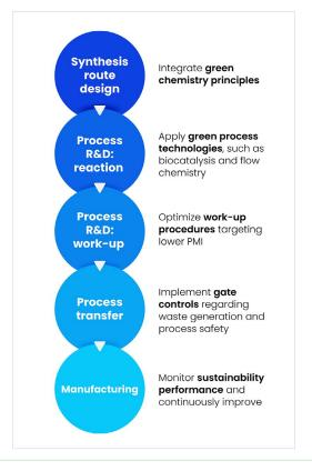
Workflow of API process development and manufacturing for greener processes
