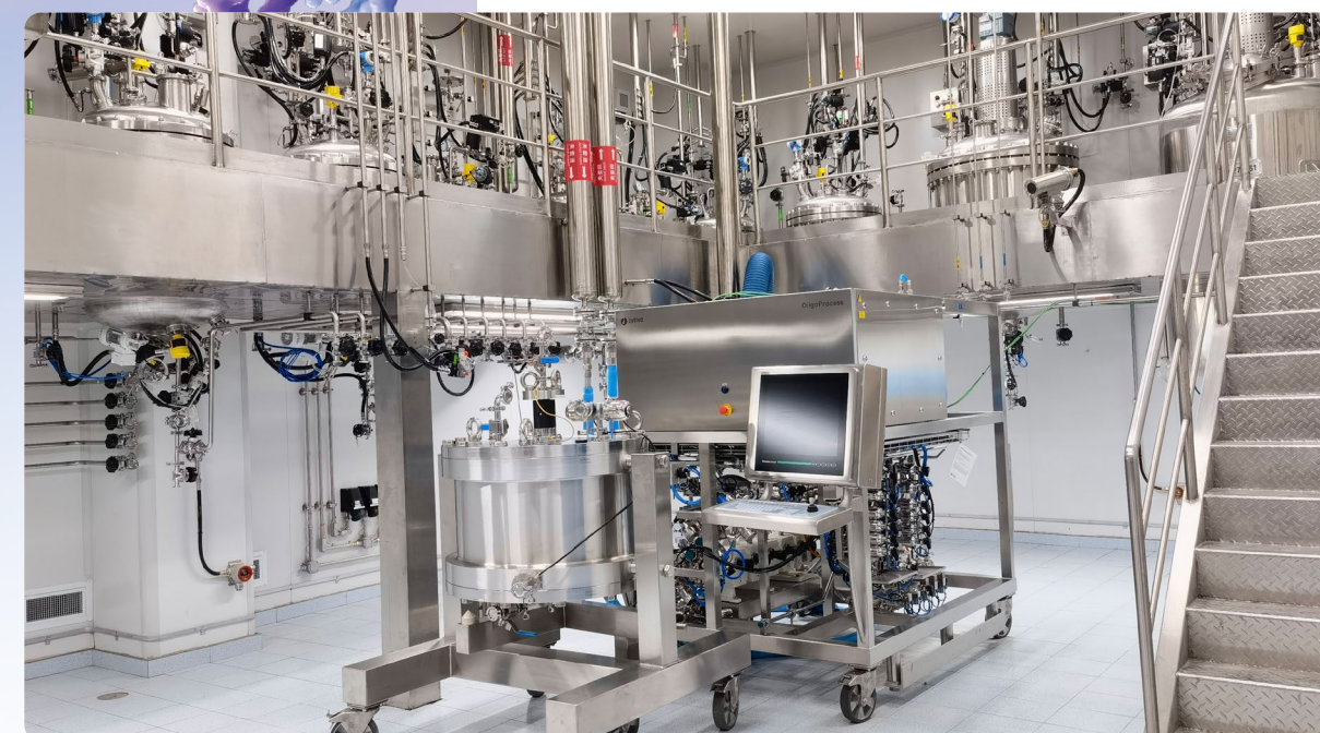
1,800 mmol synthesizer with 800 mm column
